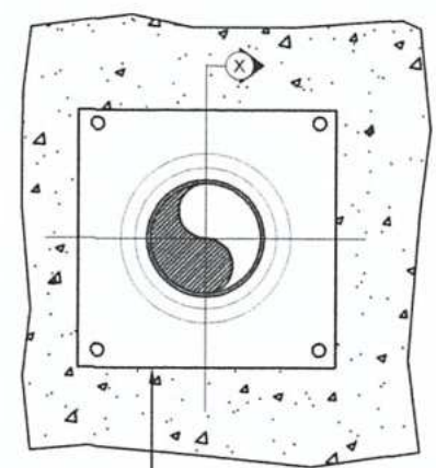
STEEL PLATE FLASHING 2 mm. THK W/EXPANSION BOLT
